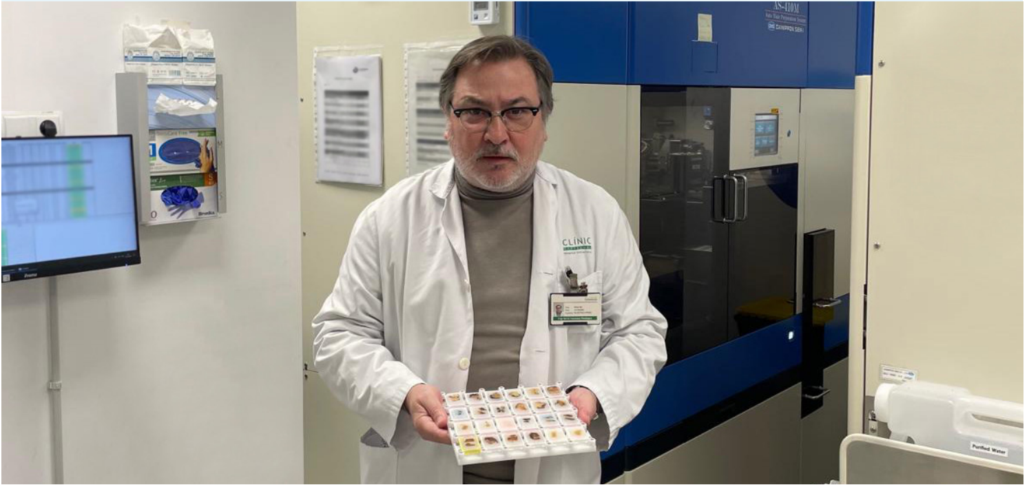
Dr. Antonio Martínez Pozo, Head of the Pathology Department at Clinic Hospital of Barcelona, holds a sample tray from the AS-410M Auto Slide Preparation System. The device has a capacity of 24 blocks per tray and a total of 96 blocks, and a full capacity of 400 slides. 🌐
