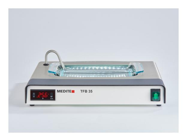
The Tissue Floatation Bath **TFB 35** is an LED-illuminated, rectangular stretching bath for paraffin sections that has been tried and tested in the routine of everyday laboratory work. The central component is the removable glass tray, under which a LED light strip is located. The light come from the rear edge under the glass tray, ensuring excellent visibility of the paraffin sections on the water surface.
