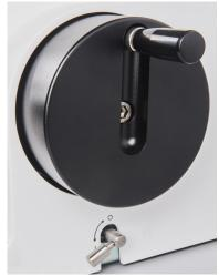
A fine adjustment mechanism is already integrated as standard feature of the specimen clamp holder. The specimen clamp can be aligned horizontally and vertically and is characterized by its particular stability. The blade holder can be easily corrected using an angle mark. The blade clamp is adjustable via grids in order to use the blade precisely and completely. It has a manual protection device.
