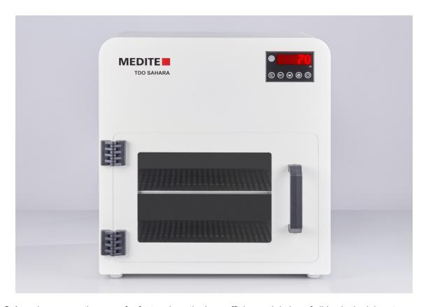
The **TDO Sahara** is a convection oven for fast and gentle deparaffining and drying of slides in the laboratory.
