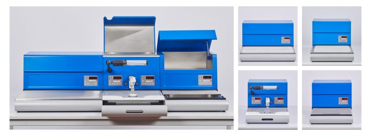
With an adjustable lamp, the work area can be illuminated as required. An optionally available magnifying glass can also be attached to the lamp. Two connections for heated forceps and six forceps slots are easily accessible around the outlet tap. The large round cooling point is in the middle. It reaches down to -5 ° C. There is also a drawer under the dispenser that collects excess paraffin during operation and can then be easily cleaned.
