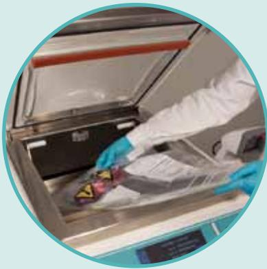
Place specimen in the vacuum bag and introduce it into the SealSAFE cavity. Close the lid.
