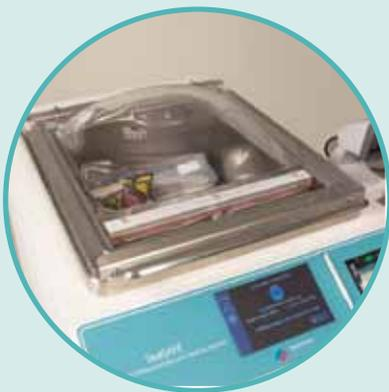
As a final step the SealSAFE vacuum seals the specimen bag. Fixative injection and sealing process are completed in the closed and ventilated cavity.
